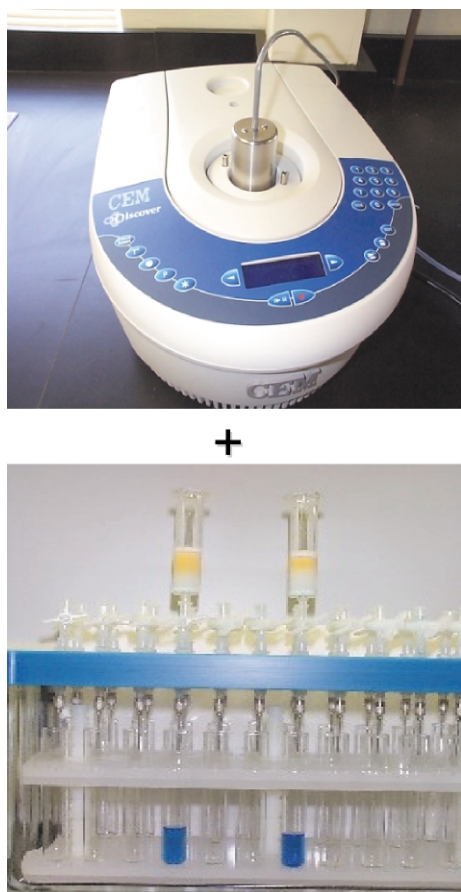
Figure 6. Fluoros synthesis with a microwave cavity (top) and an F-SPE manifold (bottom).
